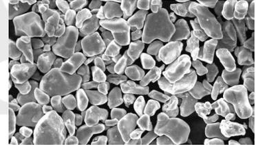
Grey powder with drop form, easy to be oxidized in the moist air.
